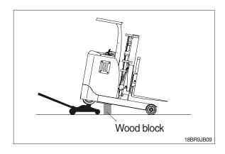
(9) Remove motor mounting bolts and motor by lifting.
