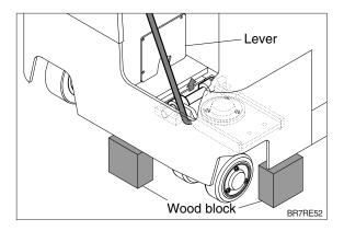
(8) Pull out the link pin from the caster suspension link.
