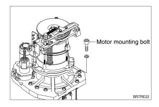
Tie wire rope around the drive motor and lift up slowly.
