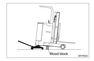
② Remove 6 flange bolts attaching the drive wheel and take off the drive wheel assembly.
