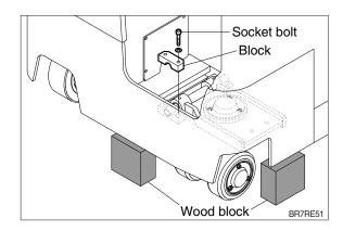
(7) Lift the caster suspension link assy with lever.
