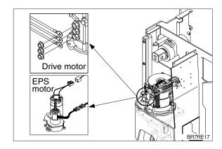
⑦ Remove bolts connecting the motor and drive unit.
