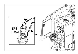
4 Loosen bolts and remove EPS motor assembly.
