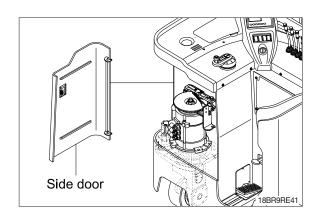
③ Remove LH cover assembly and center cover assembly.
